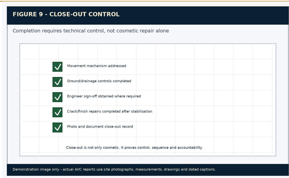
Figure 9 - Demonstration close-out control: stable repair, evidence and handover.
